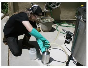
Don't forget to turn off the pump, and close all valves. Quick disconnects in sanitizer.
